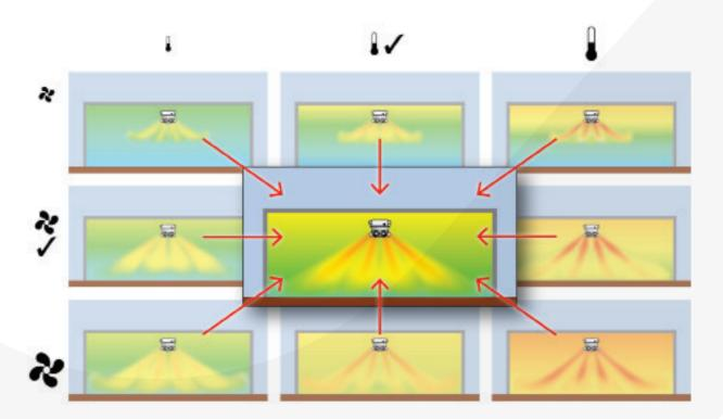
Automatically adjusting heat output and fan speed means there is always sufficient heat to warm the inducted air and there is always sufficient air speed to ensure it reaches the floor.
