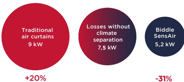
By comparing the consumption of the banking branch with and without the SensAir air curtain climate separator installed, the recorded measurements highlight energy savings of up to 29%. A traditional air curtain would lead to an increase in energy consumption of more than 20%. On average, based on the open door time of the bank branch (20%), the energy savings, achieved in the whole lobby (30m<sup>2</sup>), represent 34%.
